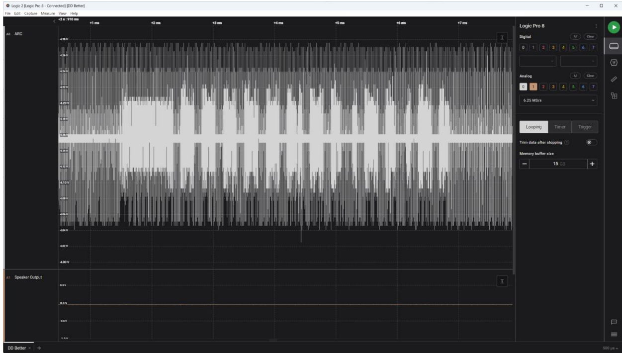
Figure 17 Dolby Digital over HDMI ARC data packet with no audio data.
