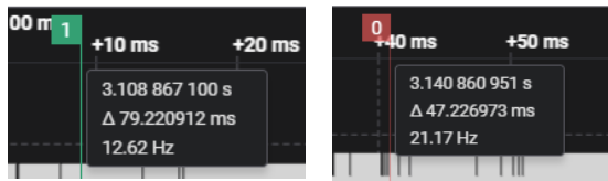
Figure 19 Marker pair 1 (green): The time between the end of the first audio packet with audio data and the rendered audio tone. Marker pair 2 (red): The time between the end of the second audio packet with audio data and the rendered audio tone.
