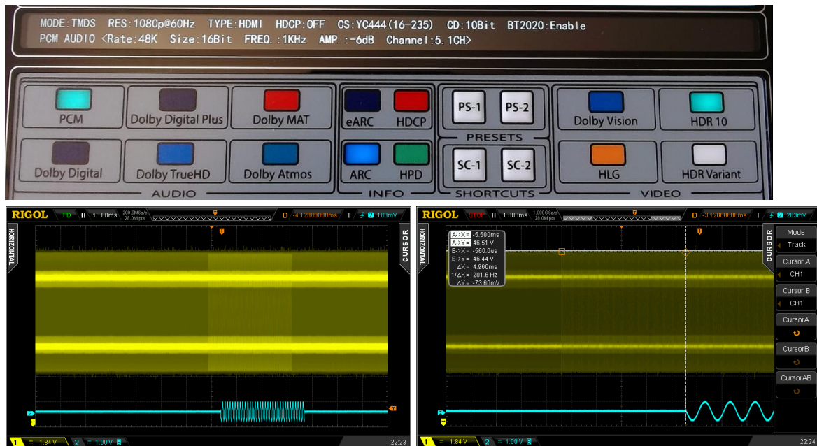
Figure 14 Top: 5.1 channel PCM M8SG ARC output configuration. Bottom: Channel 1 (yellow): HDMI TMDS Data 2 pin. Channel 2 (cyan): AV receiver speaker output.
