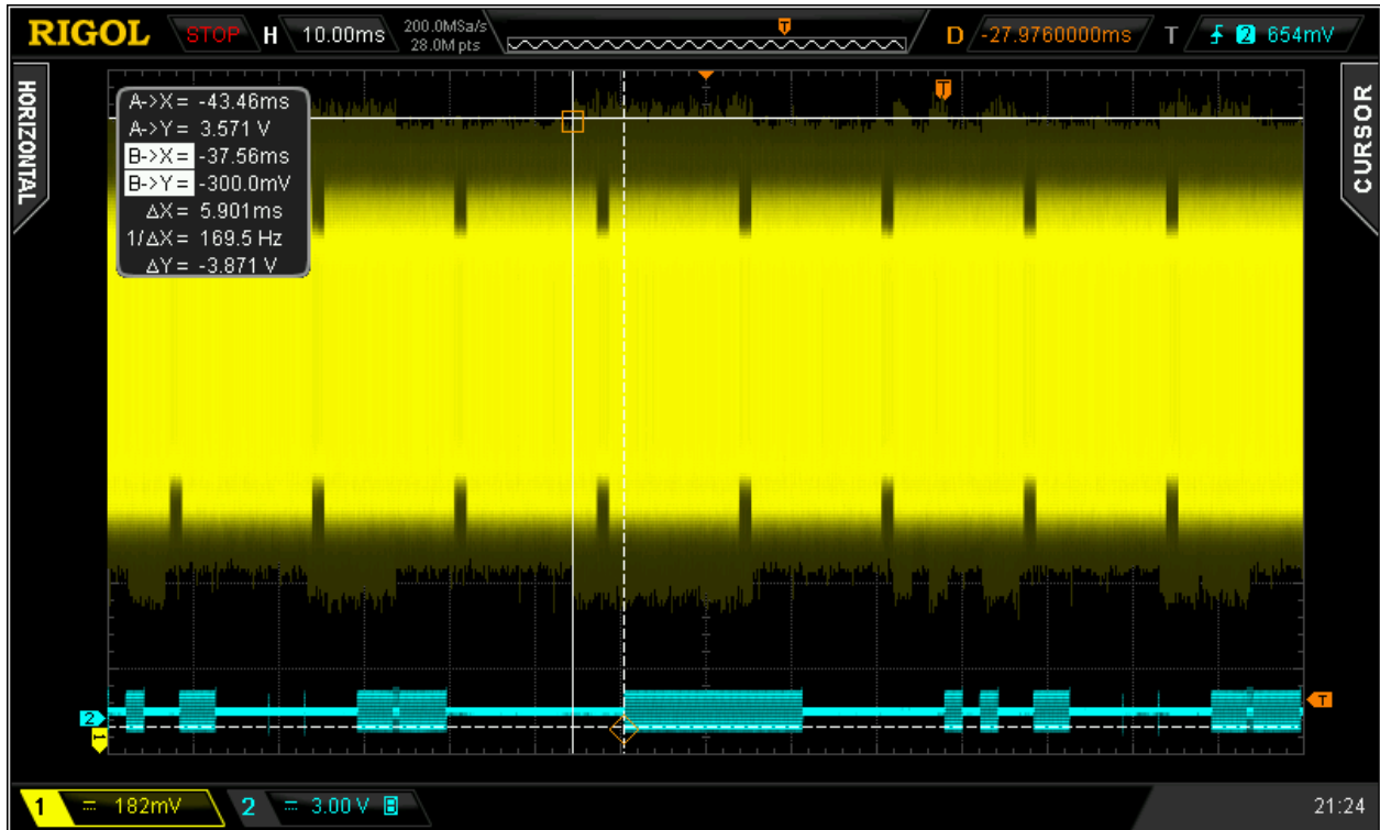
Figure 12 Surround (5.1) HDMI audio latency measurement of 5.901 ms. Channel 1 (yellow): HDMI TMDS Data 2 pin. Channel 2 (cyan): AV receiver speaker output.
