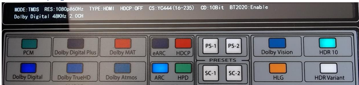
Figure 15 Dolby Digital over HDMI ARC, M8SG audio latency test pattern.
