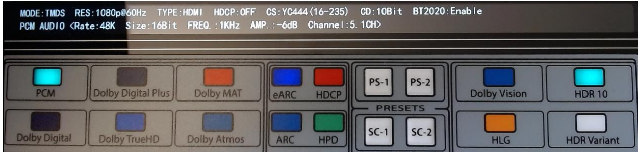
Figure 31 5.1 channel PCM M8SG eARC output configuration.
