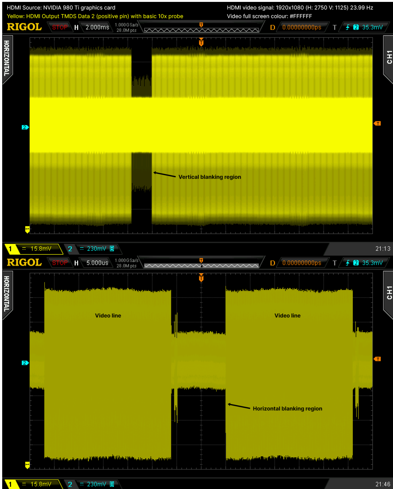
Figure 40 Top: Zoomed-out view showing vertical blanking region. Bottom: Zoomed-in view showing horizontal blanking region.
