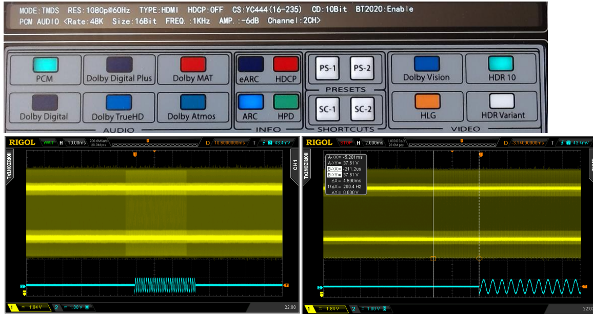
Figure 13 Top: 2 channel PCM M8SG ARC output configuration. Bottom: Channel 1 (yellow): HDMI pin 14. Channel 2 (cyan): AV receiver speaker output.
