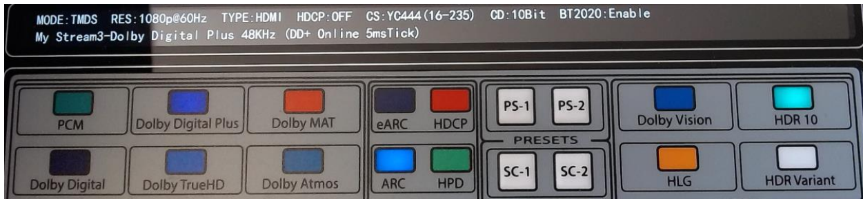
Figure 21 Dolby Digital Plus over HDMI ARC, M8SG "My Stream" custom Dolby Digital Plus E-AC3 playback on the M8SG.
