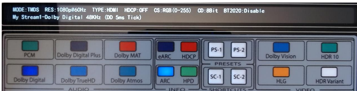
Figure 16 Dolby Digital over HDMI ARC, M8SG "My Stream" custom Dolby Digital AC3 playback on the M8SG.
