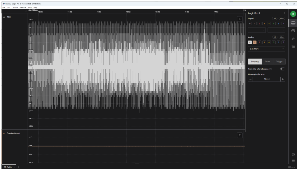
Figure 18 Dolby Digital over HDMI ARC data packet with audio data. Exactly two of these always precede the speaker output in the M8SG audio latency pattern.
